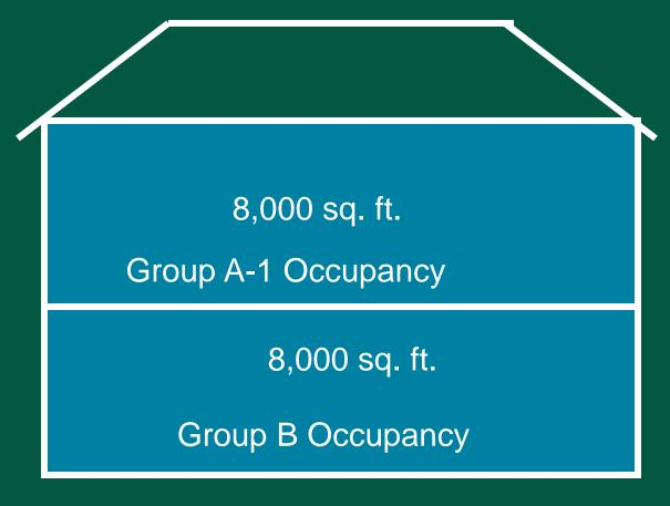
Does either floor require sprinkler protection?
